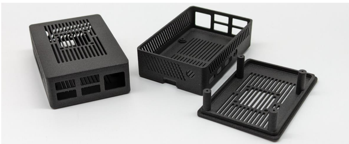
Figure 1: Photograph of PCB cases fabricated using PK ESD.
