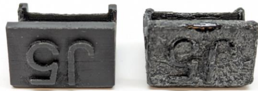
Figure 4: Conformal coating caps soaked in HumiSeal S1072 for 10 days. Formula1B (left) not affected by urethane stripper, unlike caps made with competitor ESD resin (right).
