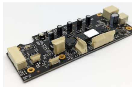
Figure 1: PCB components masked off with tape manually prior to application of conformal coating, which is labor-intensive & time-consuming.
