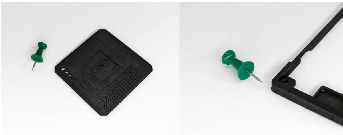
Figure 2: Example of components fabricated using DLP AM technology showcasing ability to build intricate patterns & achieve smooth surface finish.
