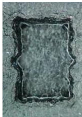
Figure 3: Microscopy image of the ESD tray pocket fabricated using SLA ESD resin. The part was rendered unusable due to poor resolution and dimensional deviations.
